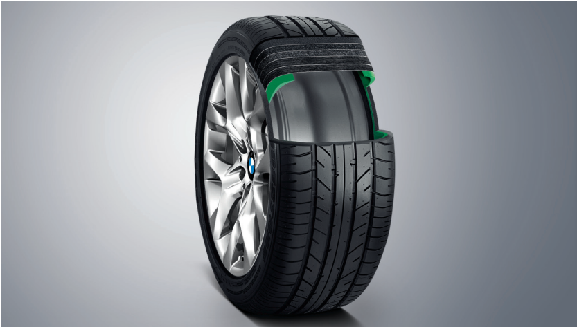
The new BMW X5 Protection VR6 has mixed tyres with emergency running properties as standard.
