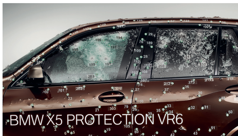
Multi-layered safety glass: the driver and passengers of the new BMW X5 Protection VR6 are protected by approximately 30-mm thick multi-layered safety glass with an internal polycarbonate splinter protection layer.(2)
