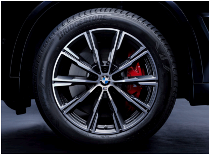
■ 20" light alloy wheels, star-spoke style 740 in M Bicolour Orbit Grey with mixed tyres and emergency running properties, diamond-polished, front wheel size 9J x 20 and 275/45 R20 tyres, rear wheel size 10.5J x 20 and 305/40 R20 tyres.
