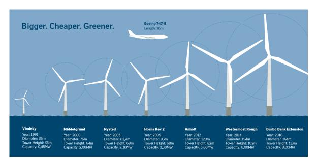
Offshore wind turbines capture the **strong and constant winds of oceans/rivers** to convert it into electricity.
